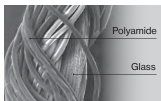
Solid construction. Core – shell – thread.
